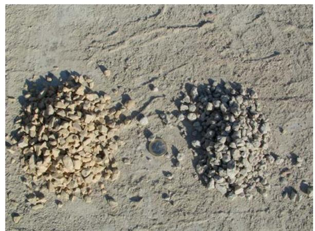
Quality of concrete of origin influences in the quality of the recycled aggregate. Recycled aggregates are better obtained from high-quality concrete. Is why a manufacturer of prestressed elements can maintain a very high level of quality recycled aggregates.
