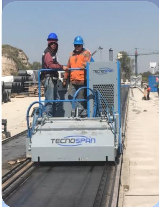
This equipment has three functions. First, clean the production track and eliminates all types of solid or liquid wastes from the work base, leaving them dry and ready for the diffusion of the desencofrant liquid and the lancing of the cords.
