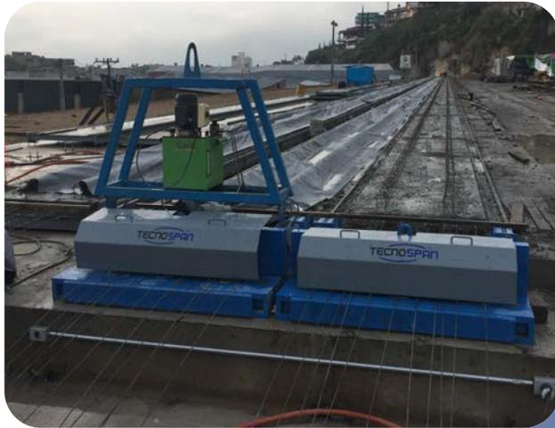
TECNOSPAN manufactures hydro-automatic devices so as to prestress steel reinforcements according to the characteristics and technical needs of each installation.
